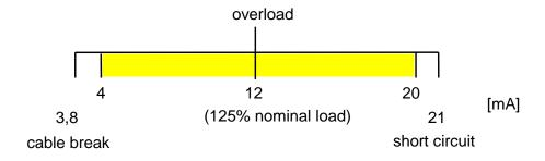
With activating the check relay a fixed signal jump of 8 mA will exceed the overload limit in every working condition. The measurement's upper limit of 20 mA however will never be reached. This makes the checking of the signal jump possible.
