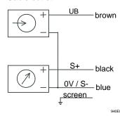
Pin configuration of connector M12x1 (4-pin) /
